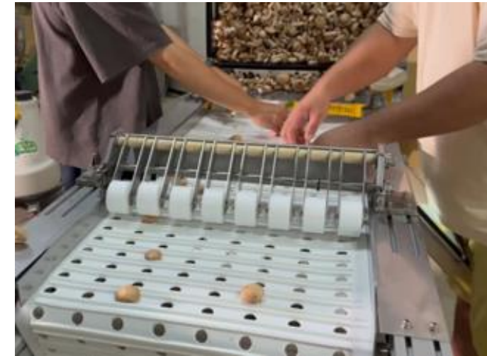
▲ semi-automatic shiitake mushroom stem-cutting machine
